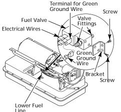
Figure 12 - Fuel Valve Replacement
